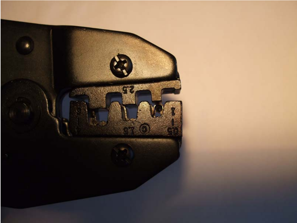
Close the crimp tool carefully until the terminal can't move anymore. (As shown)
